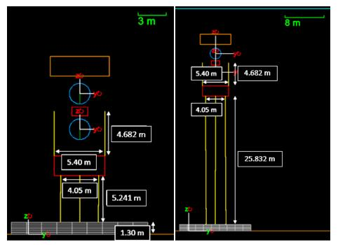
Figure 2: Layout of mooring lines and TidGen in OrcaFlex simulation model. Lines are shown in yellow. TGU is shown in blue, Upper Nacelle is shown in red.
