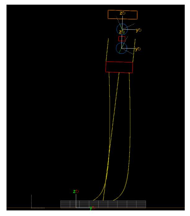
Figure 8: Screenshot of line clashing observed in Western Passage simulations
