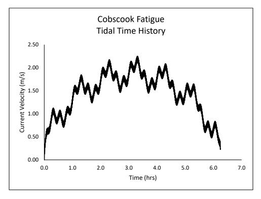
*Figure 6: Simulated current velocity of a half tide cycle, Cobscook deployment site.*
