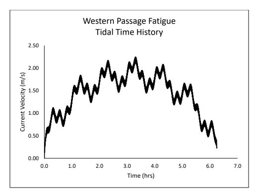
*Figure 7: Simulated current velocity of a half tide cycle, Western Passage deployment site.*
