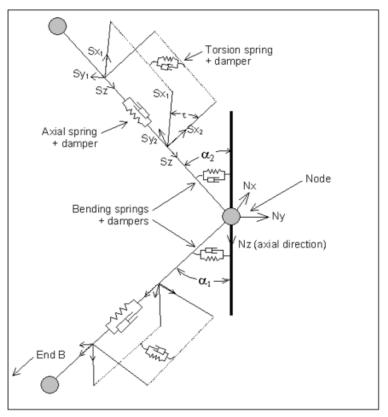
Figure 13: Representation of segment spring and damping components. Source: OrcaFlex User Manual, https://www.orcina.com/SoftwareProducts/OrcaFlex/Documentation/Help/.
