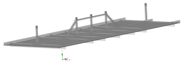
Figure 10. Steel plate, frame and padeyes embedded in concrete gravity anchor
