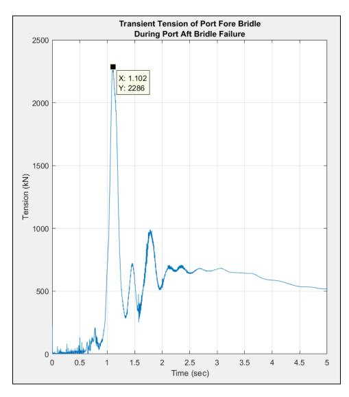
Figure 4: Simulation time history of fore bridle during aft bridle failure
