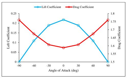
Figure 3: Lift and drag coefficients of TGU blades
